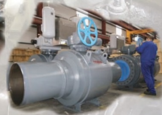
GASCO 24"-600# Fully Welded Ball Valves PUPS Gas Over Oil Actuated
